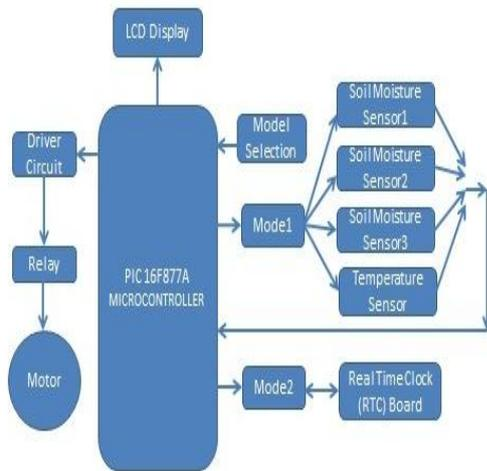
**Fig 1. Block diagram of Irrigation System**
